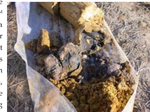
Iron distribution is seen in this core sample taken after the Ferox SM injections were completed
